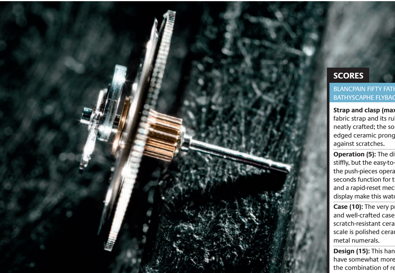
The chronograph’s vertical coupling mechanism
